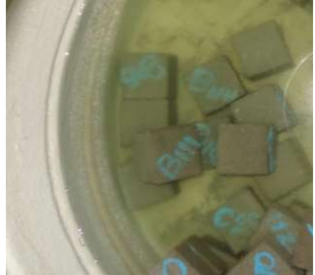
Fig 6 Water absorption test
