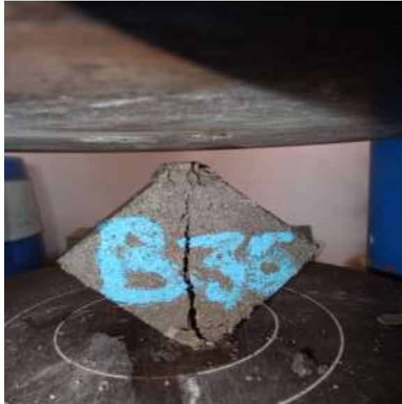
Fig 5 Setup of Splitting tensile strength
