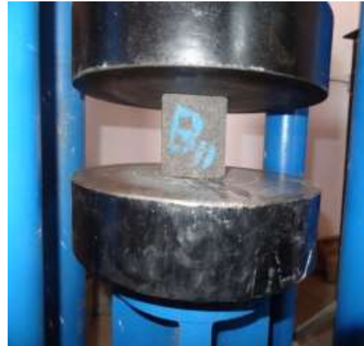
Fig 4 Setup of Compressive strength test
